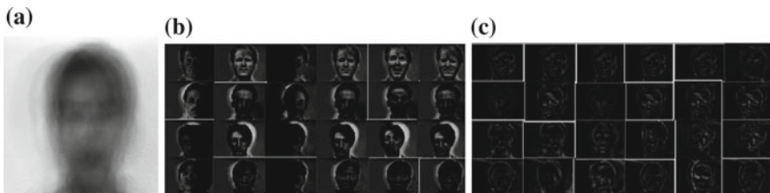
Fig. 2 a Mean face; b Normalized images of the training set; c Eigenfaces of the training set
